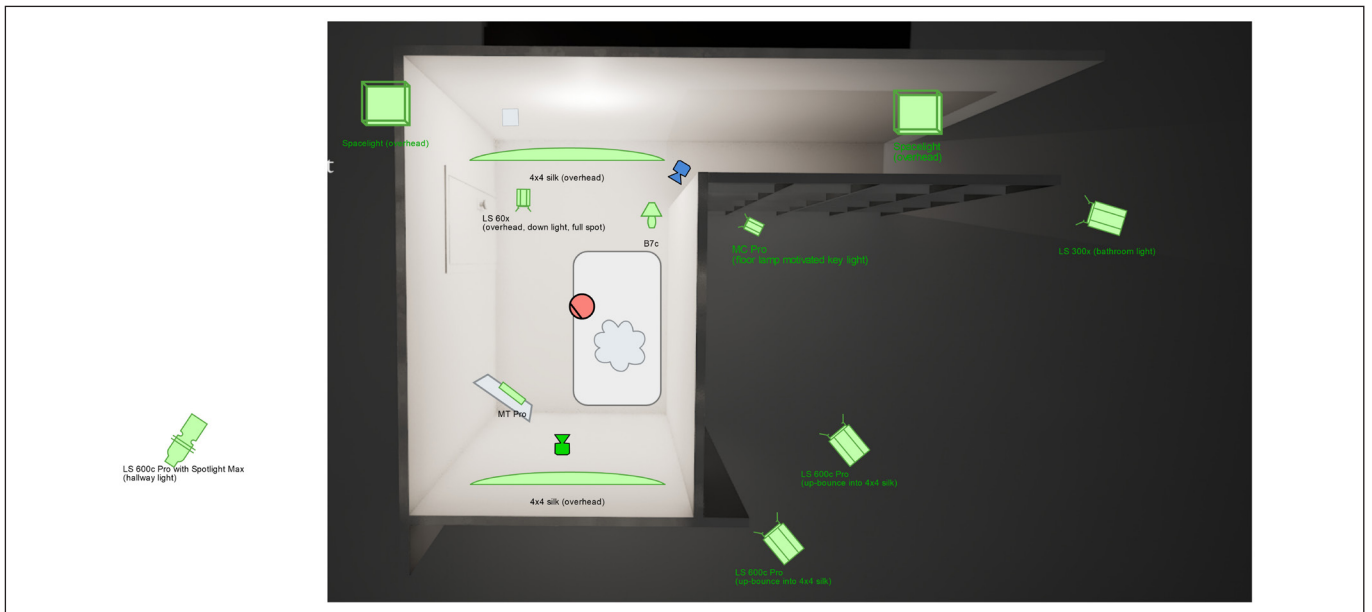
FIGURE 4. Lighting diagram illustrating a set layout with lighting fixture, diffusion, and bounce placements (2025).
