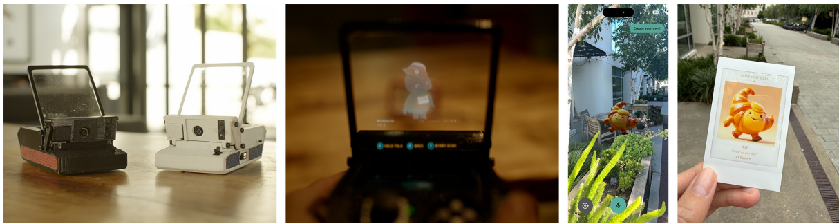
Figure 1: Lumière: a custom Polaroid-style camera (left) with an integrated Pepper's Ghost display (second left), WebAR interaction with a generated intelligent virtual agent (second right), and a printed character card artifact (right).
